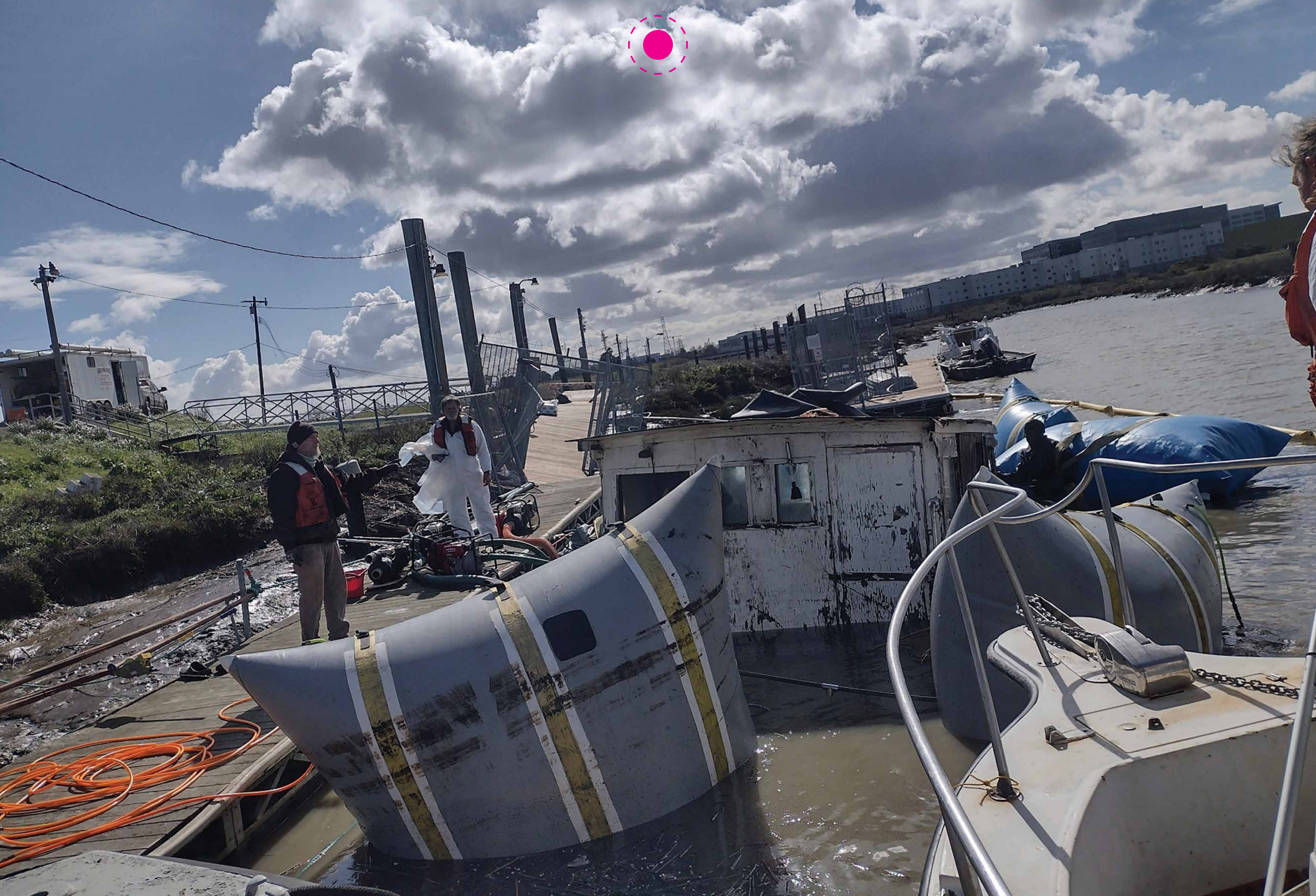
PDS raises and removes fuel from 38' steel tug sunk in Alviso Slough.
